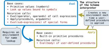
To apply a user-defined procedure, create a new frame in which formal parameters are bound to argument values, whose parent is the **env** of the procedure, then evaluate the body of the procedure in the environment that starts with this new frame.
